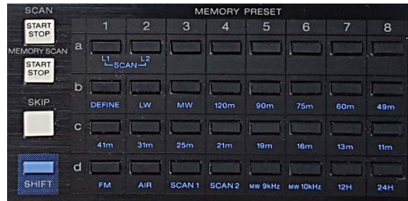
Memory matrix on the Sony ICF-2010. In conjunction with the SHIFT key, many buttons have a secondary function for scanning or band selection.
